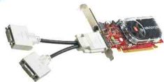
GRAPHICS - DUAL DISPLAY ADAPTER INTEL ADD2 SDVO PCIe DVI-D Adapter for dc7600 CMT, dx6100 MT DY674A
